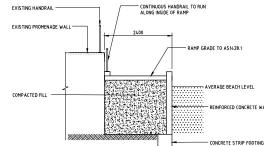
TYPICAL CROSS SECTION THROUGH PROPOSED ACCESS RAMP
