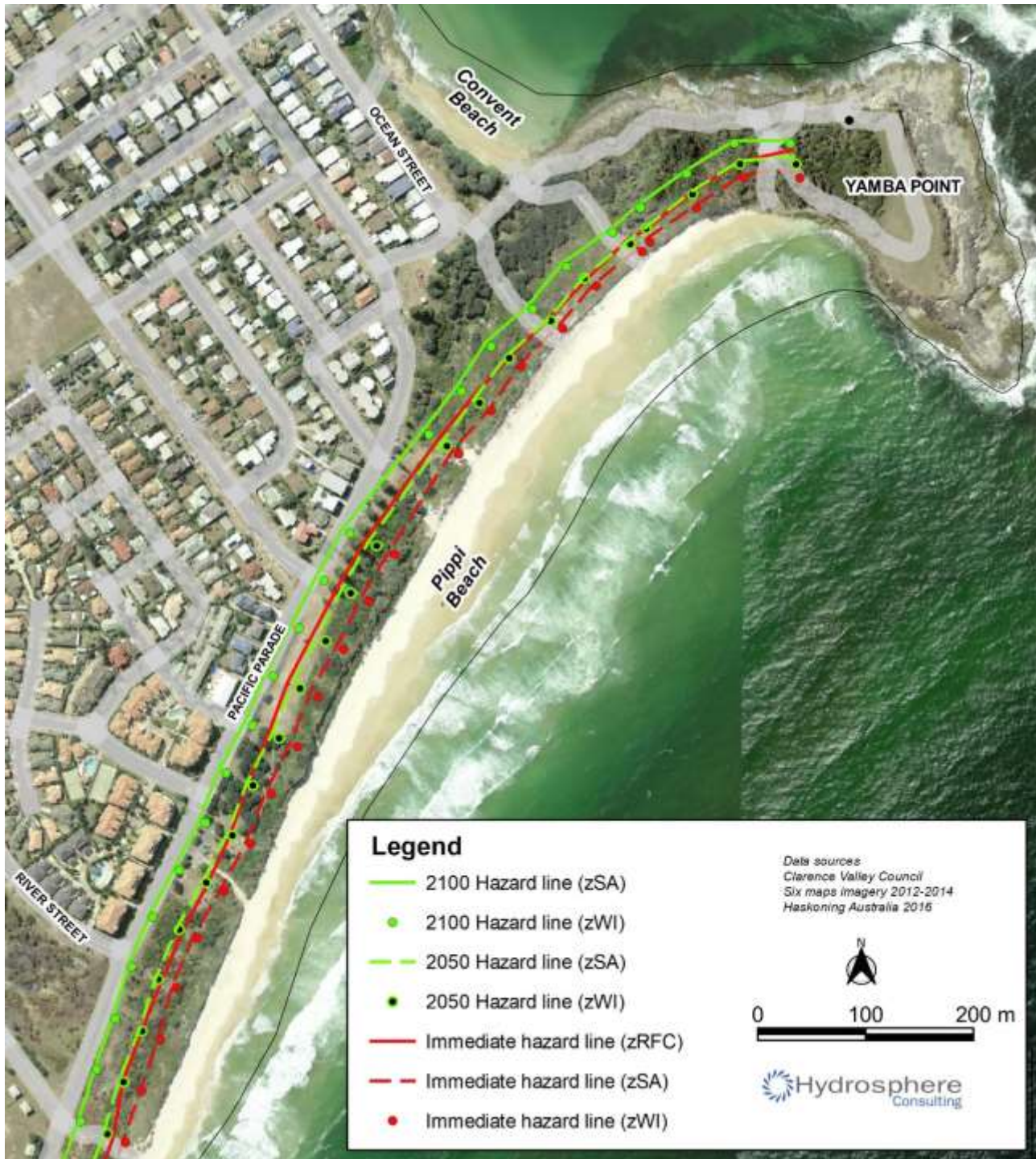
Figure 25: Coastal hazard lines for Pippi Beach - north
