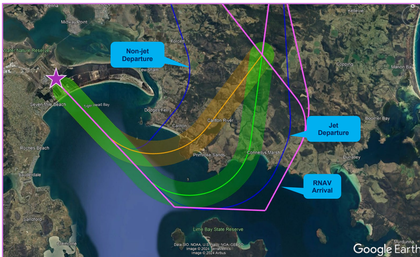
Figure 2: Current RWY 30 RNP-AR arrival flight path shown in orange , suggested change shown in green . Other existing flight paths in the area are labelled in blue . Hobart Airport is indicated by the purple star .
