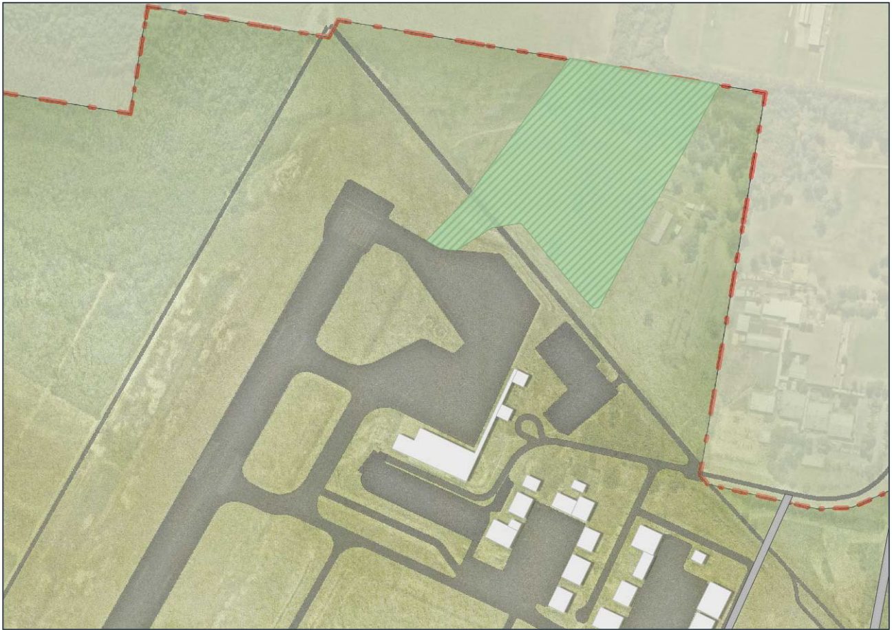
Figure 7: Hatched area showing potential location of a fifth or sixth RPT aircraft stand
