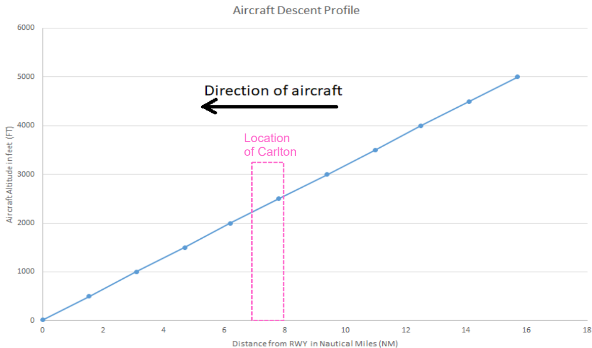
Figure 74: Example of aircraft 3 degree descent profile
