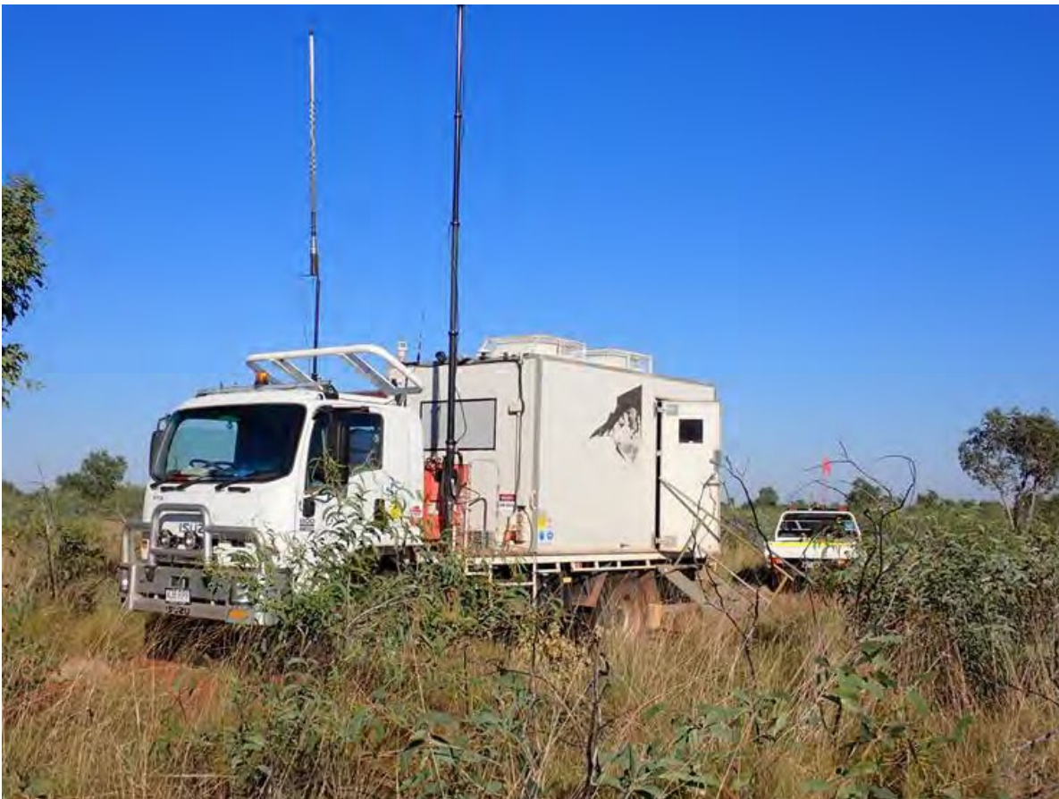
Figure 13: Data recording van used during seismic acquisition
