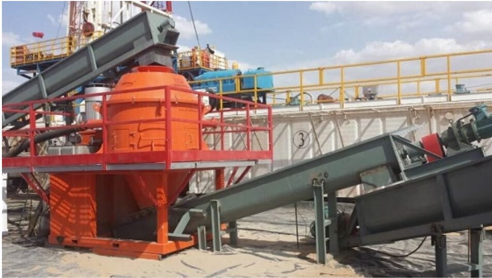
Figure 24: Example of a cuttings dryer used to recover synthetic based drilling fluids
