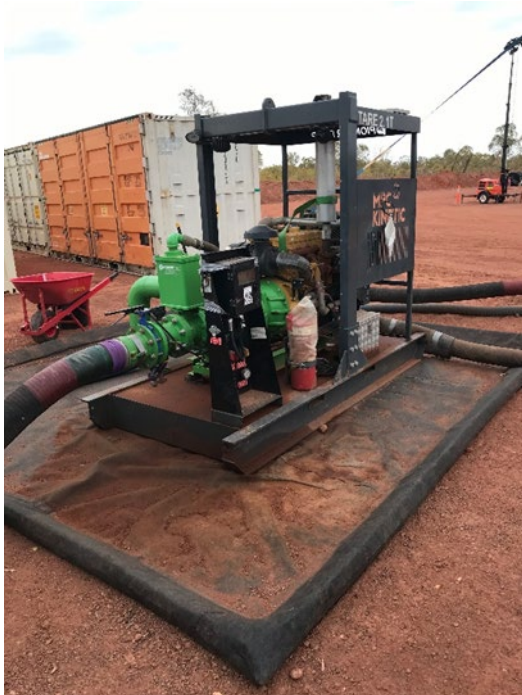
Figure 49: Examples of spill mats used to contain potential wastewater transfer spills
