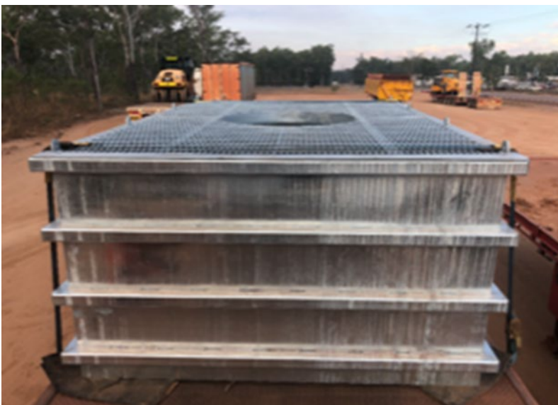
Figure 15: A cellar prior to installation
