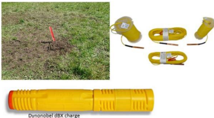
Figure 10: Example of loaded charge in hole ready for detonation and example of a charge used in dynamite seismic survey acquisition; charge length is approximately 400 – 500 mm
